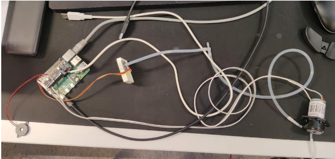
Figure 12: Testing the individual components together. Pictured is the piezo buzzer, Raspberry Pi, motor controller, pressure sensor and peristaltic pump.
