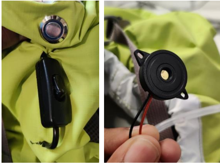
Figure 44: The pushbutton, power switch, and piezo buzzer.
