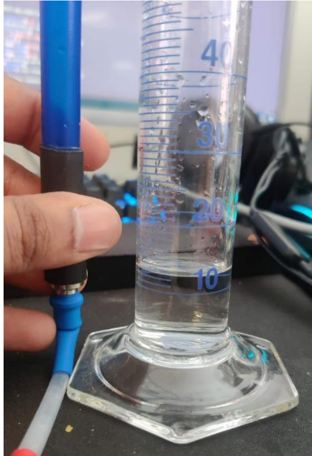
Figure 51: Measuring the tube inaccuracy.
