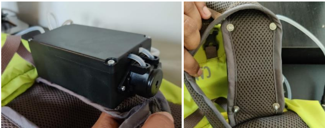
Figure 21: Peristaltic pump housing attached to CamelBak
