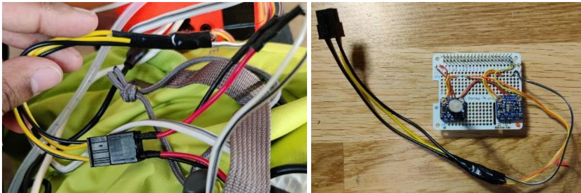
Figure 46: The Molex connector going to the pushbutton and piezo speaker.
