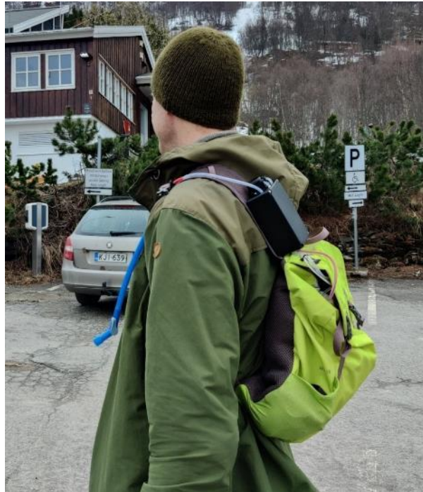
Figure 17: The implemented system. Visible are the backpack, pump housing, and drinking tube.
