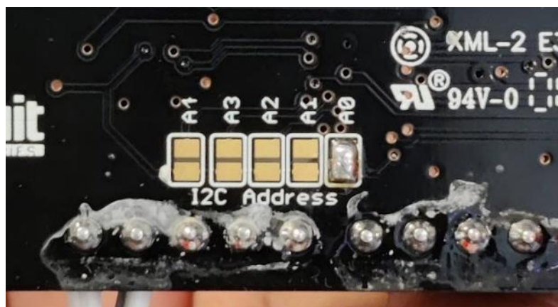
Figure 34: The I 2 C addressing PCB pads on the rear side of the motor controller.
