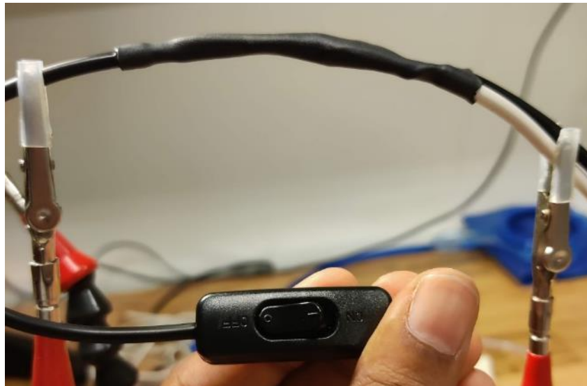
Figure 45: Modified power switch cable, connected to the RPi and motor controller.
