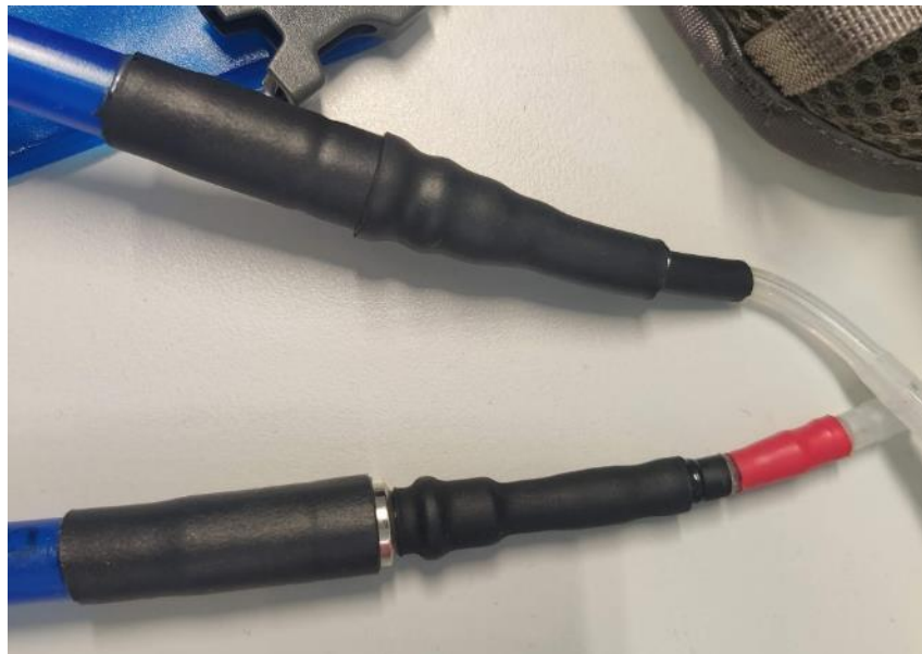
Figure 49: The heat-shrink wrapped adapters. Top: from reservoir to pump, bottom: from pump to drinking tube
