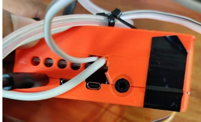
Figure 27: Modification of the side vent holes.
