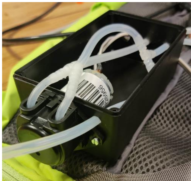
Figure 39: The peristaltic pump 14 in its enclosure
