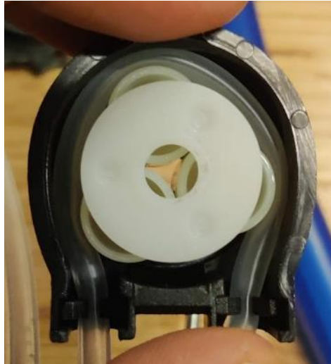
Figure 40: The pump with the plastic head removed. The three rollers are visible and are driven from the motor through a rod that goes through the center of the rollers.
