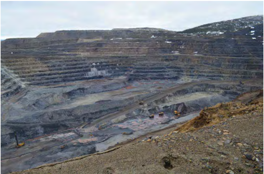
Figure 11.3 — Carol Lake mine, Labrador City, Labrador. The trucks in the photo are 7.7 metres high and typically carry 30 tons of rock per load. (Photograph by Anatolijs Venovcevs).
