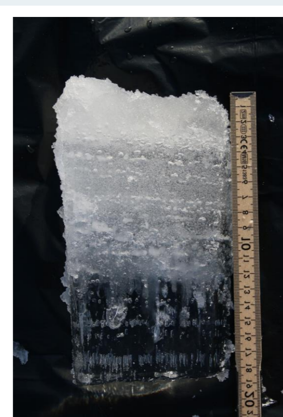
Fig. 1: Left- Ice formation in Trøsen located outside of Fjelldal, Nordland in February 2017. Right – thick section of ice. Bulk salinity of this ice was measured at 2.3 ppt, low in comparison to 'typical' sea ice which often ranges between 5 – 8 ppt. This layer of brackish ice could pose difficulties in predicting the surfacing of oil if a spill were to occur in a nearby area.
