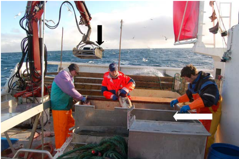
Figure 2. Governance devices: The washing and measuring bin (white arrow). Above the head of the two fishers to the left, is another cybernetic control device (black arrow), the net clearer. The net clearer has replaced the two men who hauled the nets to the stern, and thereby, structures and standardises the hauling operation. (Photo: Jahn Petter Johnsen)
