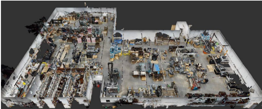
Figure 2. Areal view of the shopfloor with 3D scanning photogrammetry (a) and structure light (b) type
