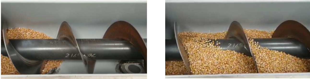
Figure 23. Experiment to show behavior of materials in a screw conveyor.
