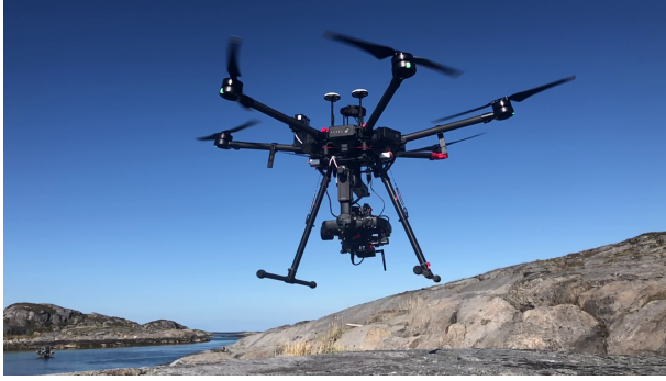
Fig. 1: DJI Matrice 600 Pro drone carrying gimbal with Resonon Pika L hyperspectral camera.
