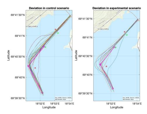
**Figure 4**: The deviation between the planned route and the sailed route is presented both in the control and experimental scenarios. Note that the result only presents the greatest deviation occurring between the point at which participants began turning and the point where they aimed to cross the narrow bridge.
