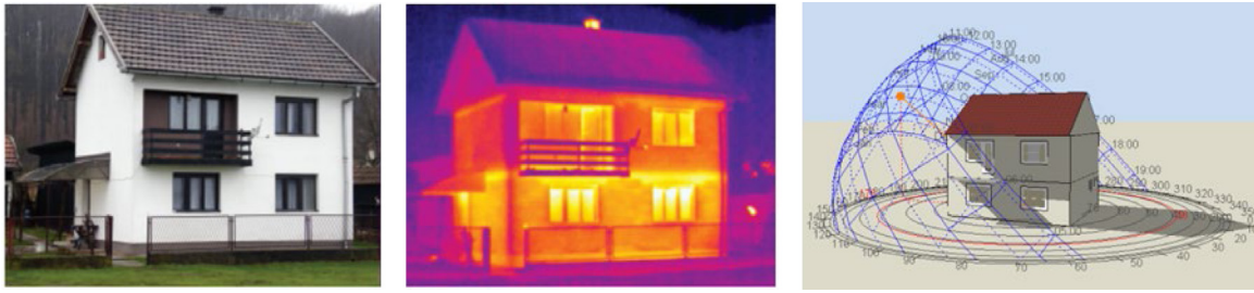
Fig. 1. (a) Visual and thermographic presentation of the selected building, (b) DesignBuilder model.
