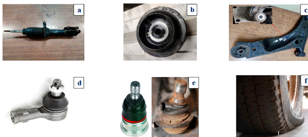
Figure 4. (a) strut mount failure (b) strut external damage (c) lower arm bush worn out (d) lower arm ball joint fault (e) strut worn out and (f) low tire pressure.
