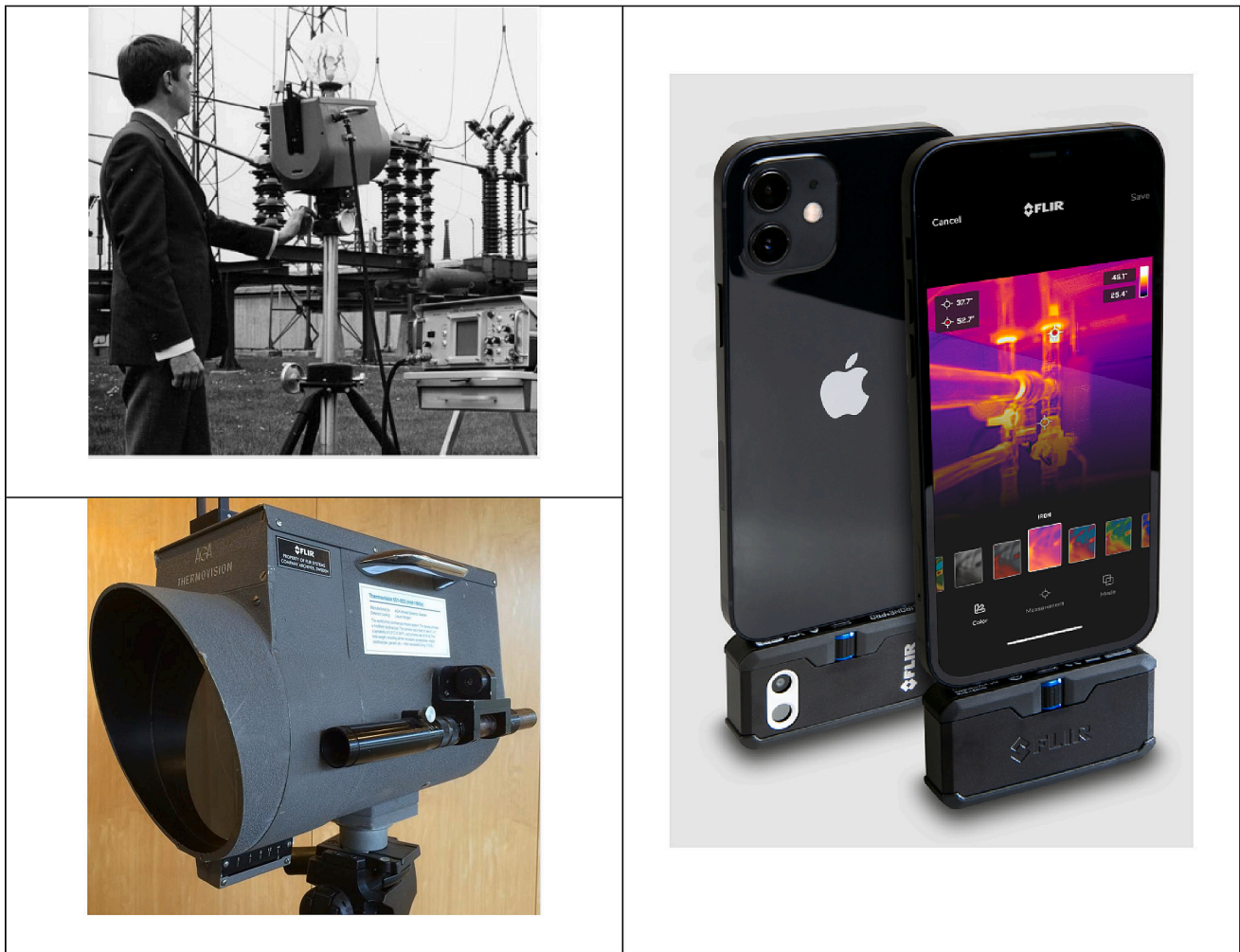
Fig. 4. Technological evolution of thermal infrared technology: pictures on the left display AGA Thermovision-661 IR camera developed in 1969 in Sweden. This thermal IR camera with a Field of View (FOV) of 5^{\circ} \times 5^{\circ} , thermal sensitivity of 0.2^{\circ} \text{C} and mass of around 25 kg needed to be supported by oscilloscope (20 kg) and tripod stand (15 kg) and cooled using 10 l cryogenic cooler (liquified Nitrogen) powered by 220 VAC generator. Picture on the right shows a modern portable FLIR ONE Pro ® thermal IR camera released in 2017. This handy camera weighing merely 36.5 g can be connected to smartphone and features 50^{\circ} \times 43^{\circ} FOV with thermal sensitivity of 0.1^{\circ} \text{C} (100 mK) (Gromicko and McKenna, 2022; AGA Thermovision, AGA Museum, Emmen, Netherlands, n.d.; Teledyne, 2023).
