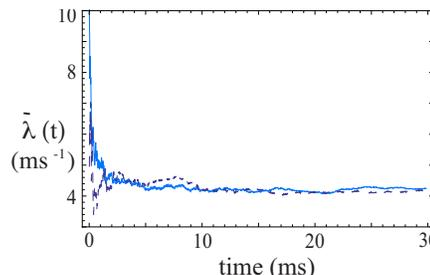
FIG. 5. (Color online) Computation of growth rate  $\bar{\lambda}(t)$  from diffusionless Lorenz model signal (dashed) and low-pass filtered electron density signal in light blue (dark gray). The limit of large  $t$  yields the Lyapunov exponent  $\lambda$ .
