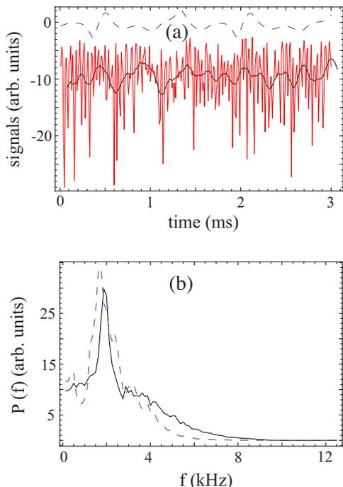
FIG. 3. (Color online) (a) Upper dashed trace is the signal for the profile gradient variable  $z$  in the diffusionless Lorenz equations for  $R=3.3$ . The lower rapidly fluctuating red (gray) trace is the electron density fluctuation signal at  $x=12$  cm, along with the black signal filtered by a moving average. (b) Spectral power density for diffusionless Lorenz signal (dashed) and for low-pass filtered electron density signal (black).
