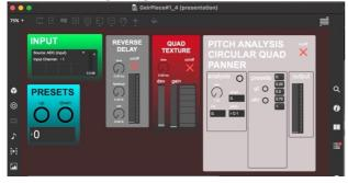
Figure 3. Software modules example in Max/MSP
