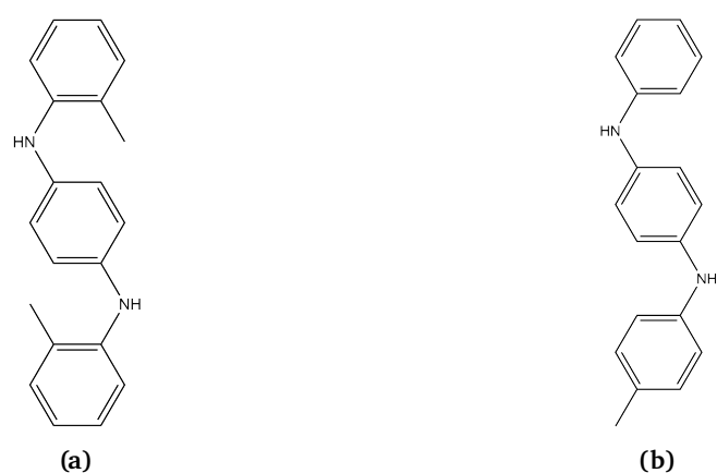
Figure 4.1: Molecular structures of DTPD (a) and TPPD (b).
