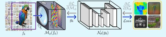
Fig. 3. E2E scheme where the COI system is modeled as optical layers. In training, a set of images passes through the optical system, obtaining the projected measurements that enter the computational decoder producing an output for an arbitrary task. The estimated task error is propagated from the output of the decoder to the optical layer, updating the weights of the decoder and the optical system.
