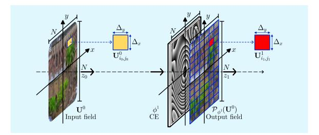
Fig. 2. Visual representation of the discretized propagation and the modulation of a CE in an optical layer. The incident field  $\mathbf{U}_0$  is propagated and then modulated by the CE ( $\phi$ ) where the field immediately after the  $i_1, j_1$  pixel (or neuron) is given by  $\mathbf{U}_{i_1, j_1}^1$ .
