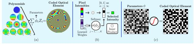
Fig. 4. Parametrization of different optical elements, (a) DOE, where the trainable parameters are the coefficients associated with Zernike polynomial  $Z_i$  (b) color filters, where the parameters are a vector of weights that select one of the available filters, and (c) coded aperture, where the trainable parameter is a continuous variable.
