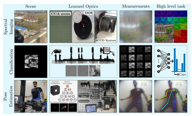
Fig. 8. Three representative optical encoding and computational decoding applications that employ E2E optimization, (Top) spectral imaging, (Middle) image classification, and (Bottom) human pose estimation.
