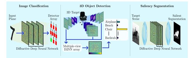
Fig. 9. Three types of all-optical applications of D2NNs for image classification (left), 3D object detection using multi-view D2NNs (middle), saliency segmentation by placing the D2NN at the Fourier plane of the 4-f system (right).
