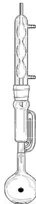
Figure 12: Soxhlet extraction apparatus. Photo credit: Sigmaaldrich.com
