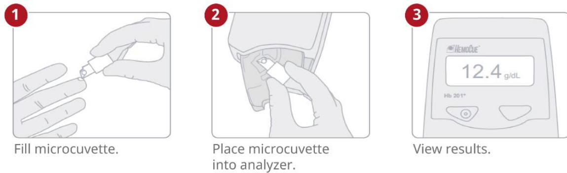
Figure 13: Illustration of measuring the haemoglobin using Hemocue Hb 201+ Analyzer. First one fills the microcuvette with 10 \mu L blood and places the microcuvette into the analyser. The analyser measure the haemoglobin levels (g/dL) and shows the levels on the display (Hemocue).
