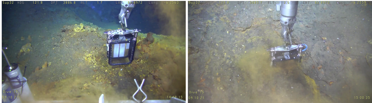
Figure 3. Video stills capturing the moment before BlaC01 is thrust into the sediments on the left, and the on the right BlaC03 has penetrated into the seabed.
