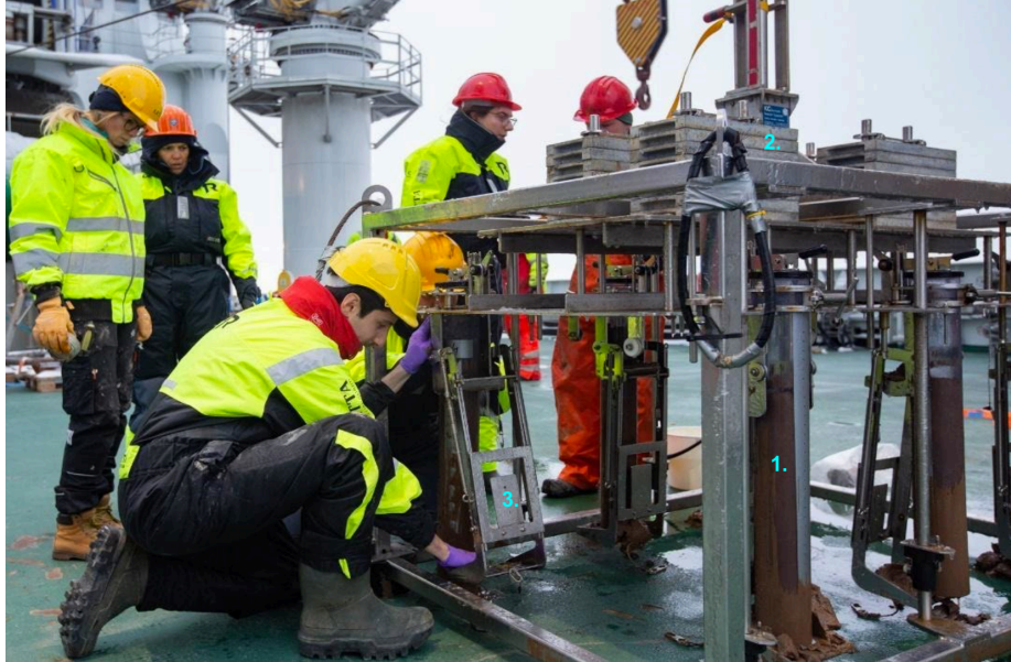
Figure 4. KC Denmark DK8000 on the ship deck after a successfully retrieving MC-148. 1. Plastic liners in the MC, 2. lead weights to provide gravitational force into the sediments, 3. core catchers to retain sediment upon retrieval. Edited after (Bunz & Ramirez-Llodra, 2021).
