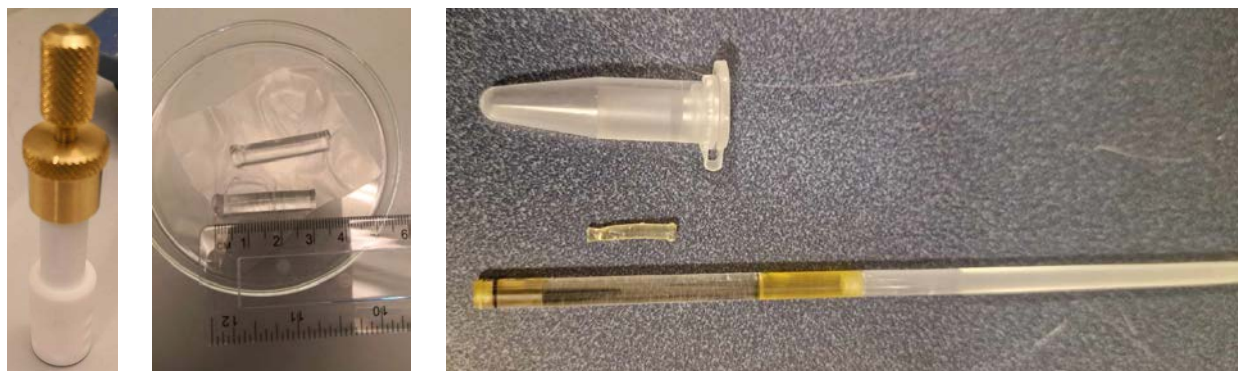
Figure 17. (Left) The New Era gel transfer set used to transfer the PAA gel from the casting/swelling chamber, in the middle, to the open-ended NMR tube. (Middle) Two sticks of cast PAA gels after washing, ready for drying on parafilm. (Right) Dried PAA gel and stretched PAA gel in an open-ended NMR tube with a bottom plug and top rod, Eppendorf tube for scale.
