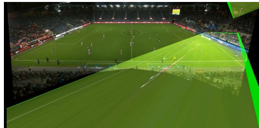
Figure 7. Warped image using homography with low accuracy.
