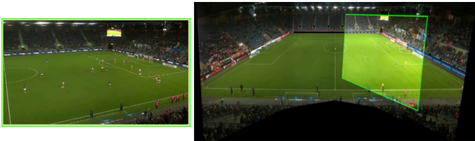
Figure 2.2: Perspective project of frame in video clip to panorama image.
