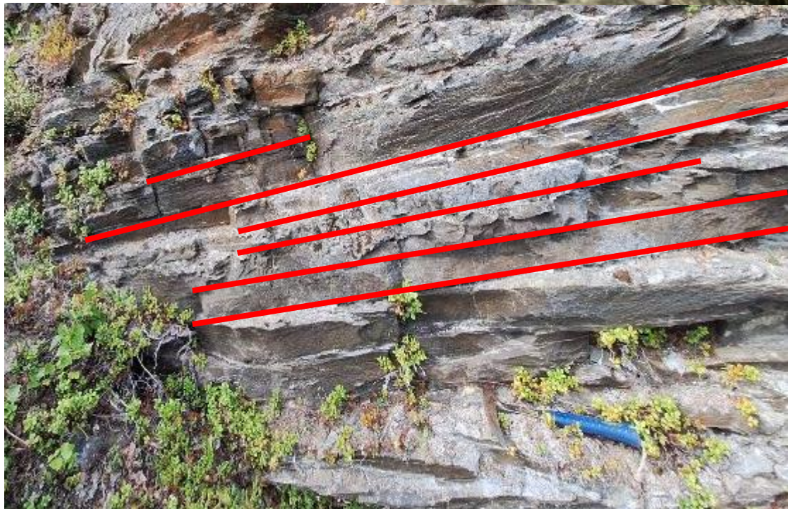
Figure 33 Foliation set projection; Foliation expressed in the field (picture top right taken by NGU 14/08/23)
