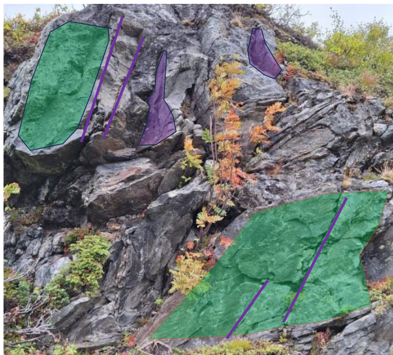
Figure 36 Joint set 2 (green) & 3 (purple) at location 10
