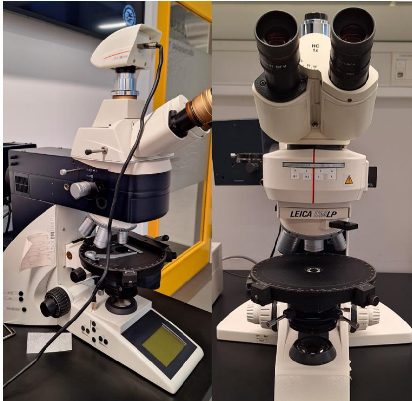
Figure 22 left Leica DM 4500 P microscope; right Leica DMLP microscope
