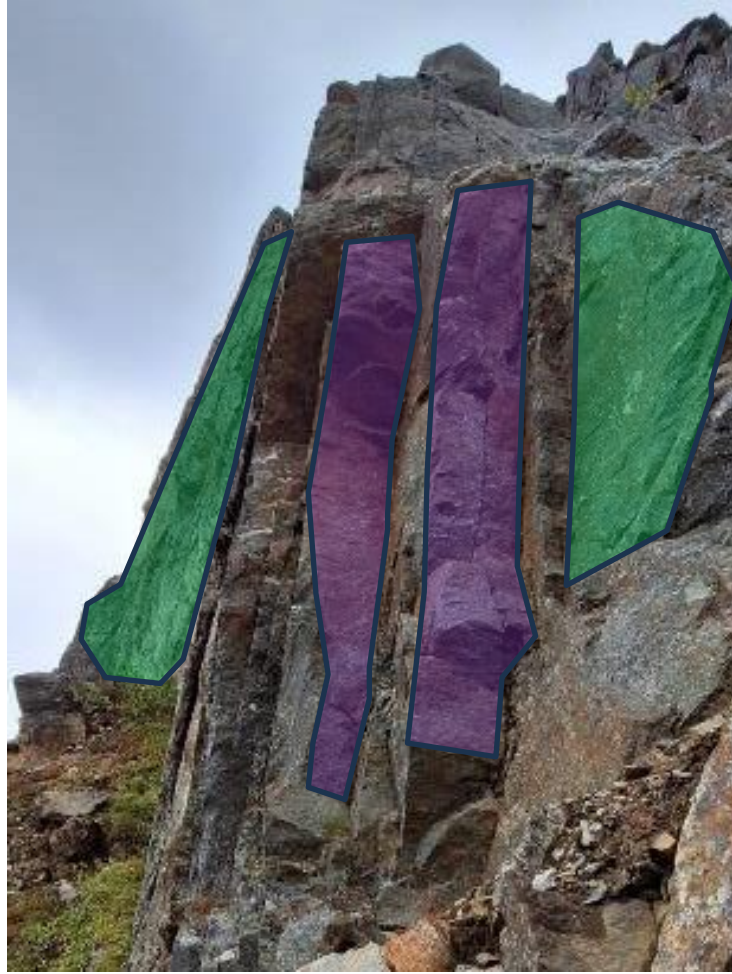
Figure 37 Joint set 2 (green) & 3 (purple) at location 13
