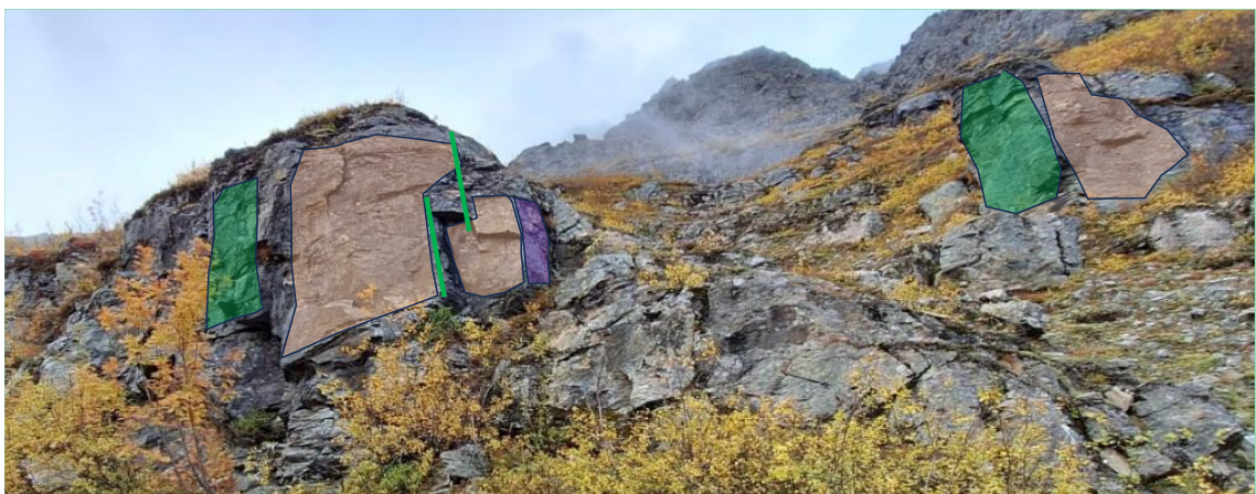
Figure 38 Joint set 1 (orange), 2 (green) & 3 (purple) at location 16
