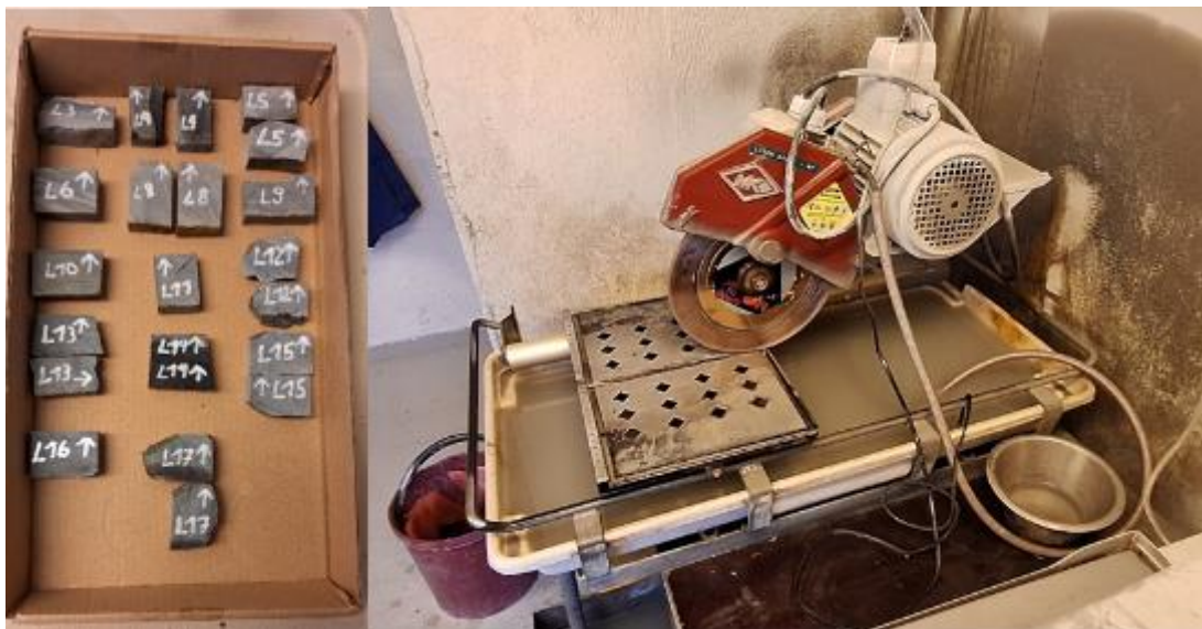
Figure 21 Sample blocks (left), Rock saw used (right)
