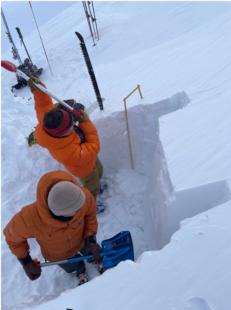
Figure 4.1.5: Shaping the snow pit to conduct an ECT-test, in collaboration with Skred AS at one of their weekly snow cover surveys. Picture taken by the author's field assistant nr. 2 of 2: Vilde Edvardsen Hansen.
