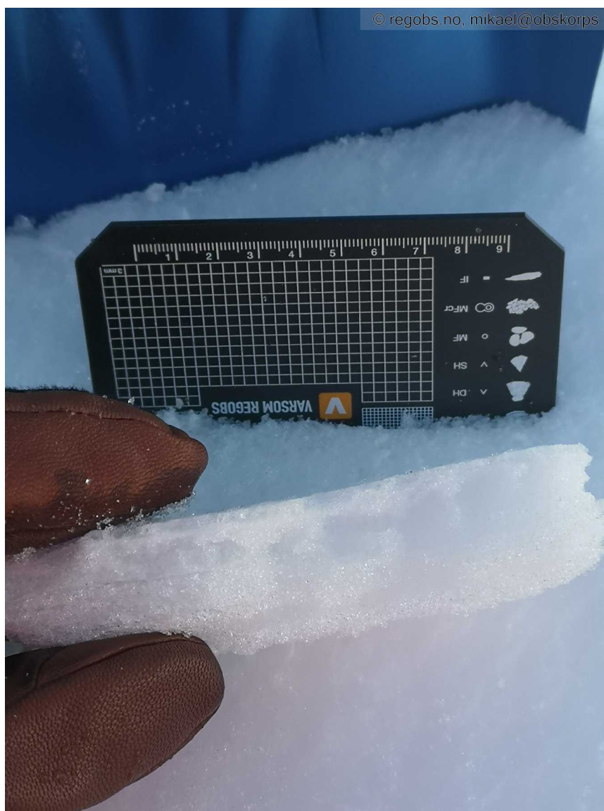
Figure 5.3.6: Upper part of the crusted base, which covers most of the plateau. The layers of crust and melt forms can be seen here. This is a cross-section related to snow pit survey part C in Fig. 5.3.7.
