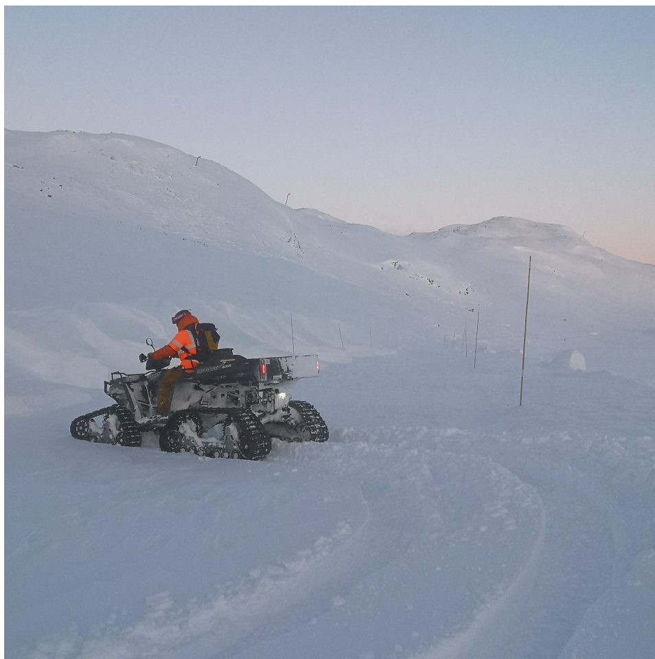
Figure 3.1.7: The snow covered road of County Road 53 Tyin-Årdal after a snowdrift event. Subsequent avalanche control and snow plowing were conducted later the same day. Avalanche towers Støl 1 & 2 can be seen in the background. Picture taken in the north-west direction by the author 21.02.2023.
