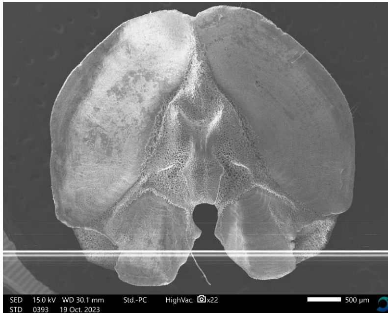
Figure 7. Example of charging artefacts (the white horizontal line) obscuring part of an Ophiopleura borealis ossicle in an SEM image at 15 kV.
