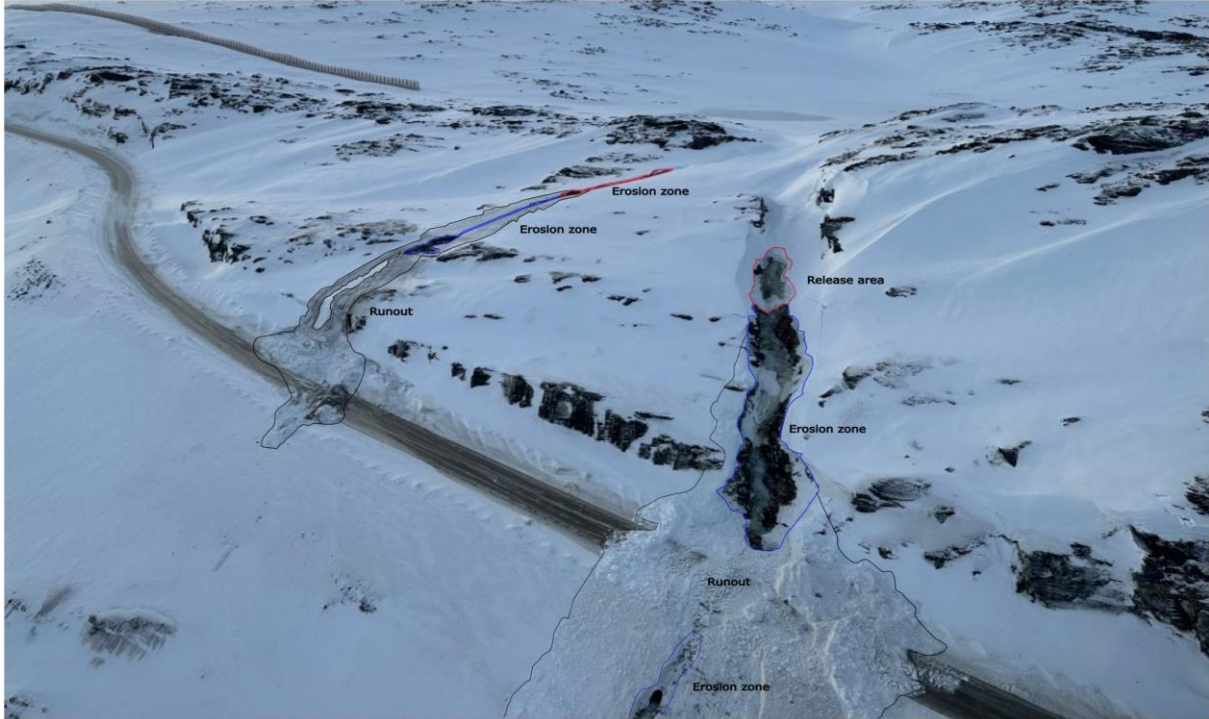
Figure 18: Documentation of Fv 889 Bakfjorddalen events. The identified release areas are outlined in red, erosion zone in blue and runout in black. On the flat area above the releases is the grey-blue area illustrating saturated snow marked with a light blue outline.
