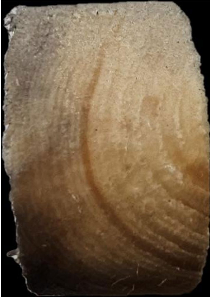
Figure 18 CW sample oriented in the same direction as the profile with the bark to the left at z=0 mm and pith to the right at z=0,9 mm
