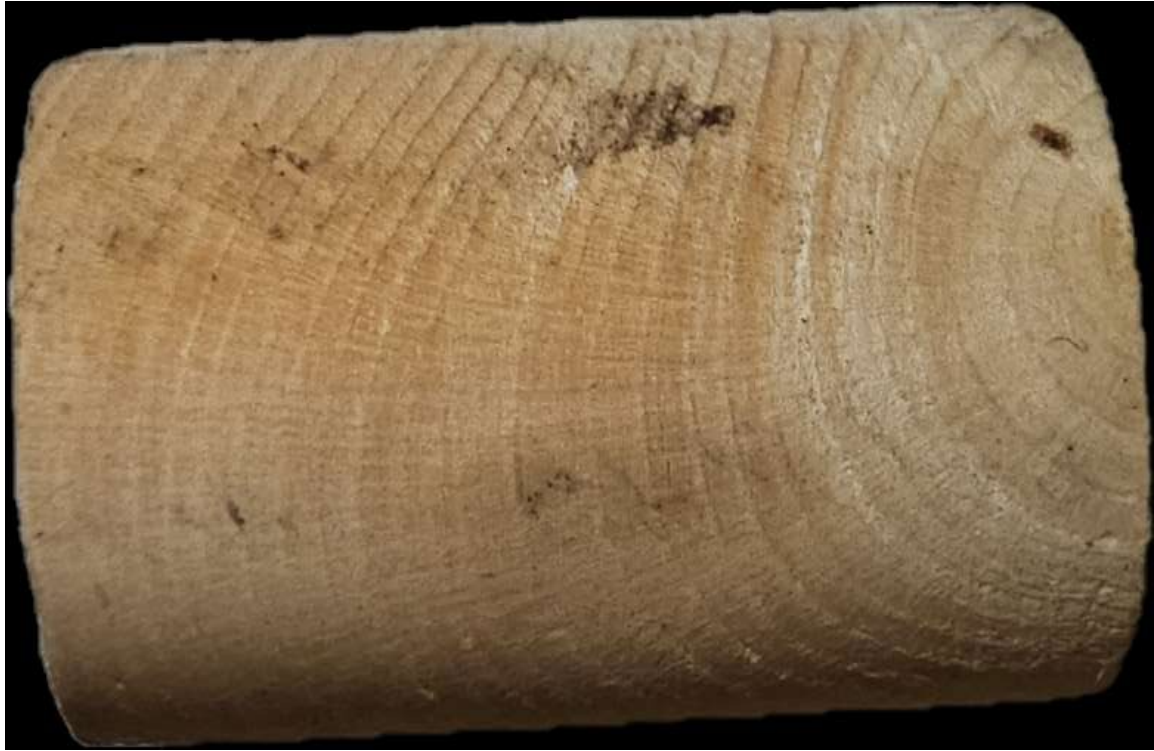
Figure 15 OW sample oriented in the same direction as the profile with the bark to the left at z=0 mm and pith to the right at z=21,5 mm
