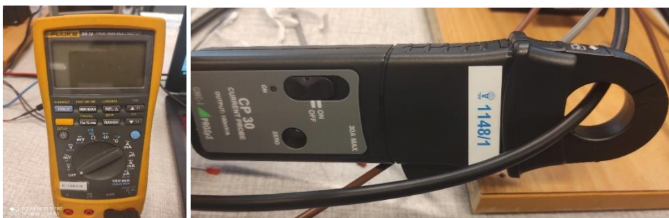
Figure 19: Equipment for current and voltage recovery
