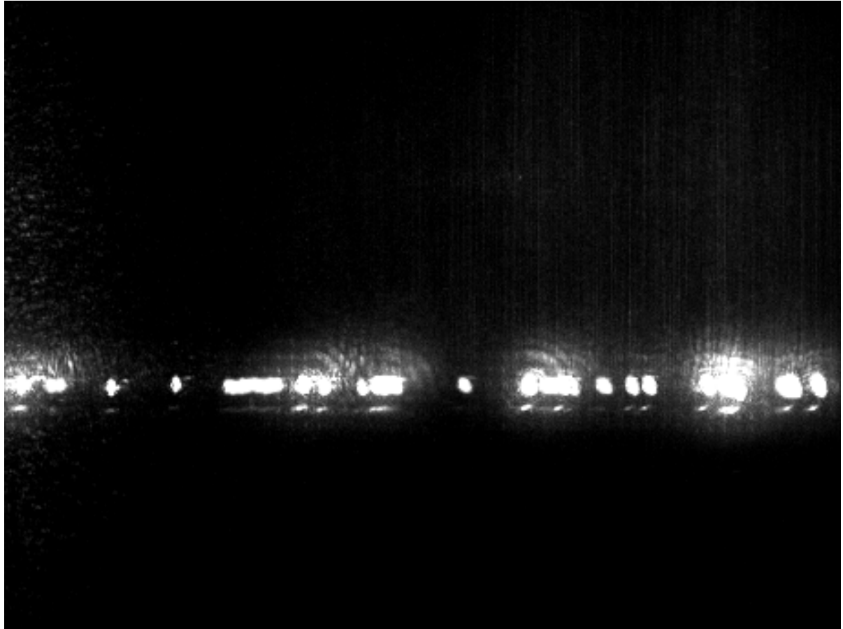
Figure 6.2: Nanoparticle with diameter 500nm trapped on waveguide (x20,DF, 200mW)
