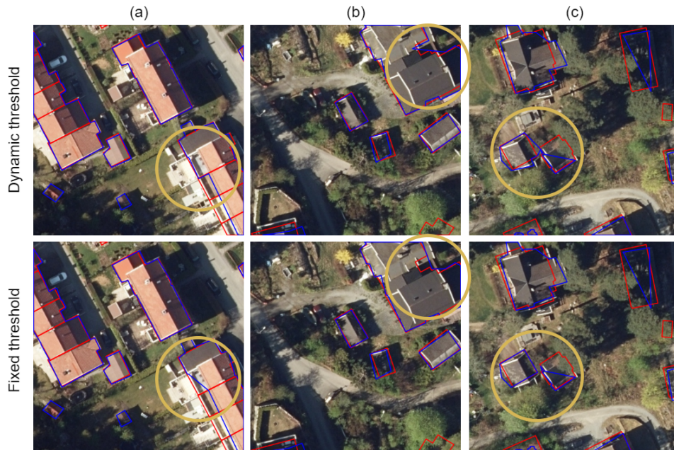
Figure 8.10: Qualitative analysis of our dynamic threshold selection algorithm. The top rows are examples where the dynamic thresholds are used, while the bottom row shows the fixed threshold. The predictions are shown in blue, while the red polygons represent the ground truth annotations. Columns (a) and (b) highlight cases where our method improves the quality of the polygon by being able to select vertices at a greater distance if the model is uncertain in the placement of the vertex. Column (c) highlights a failure case, where the vertices between two buildings are too close, causing the polygon of the left building to select an additional polygon which should not have been there.
