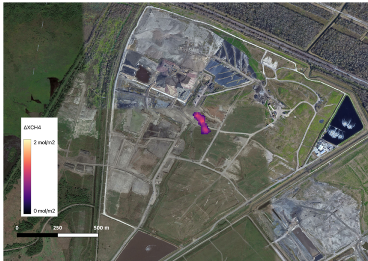
Figure 7.11 Possible methane plume December 18 th , 2022. The background image is provided by Google Earth.
