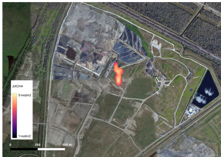
Figure 7.8 Possible methane plume April 27 th , 2022. The background image is provided by Google Earth.
