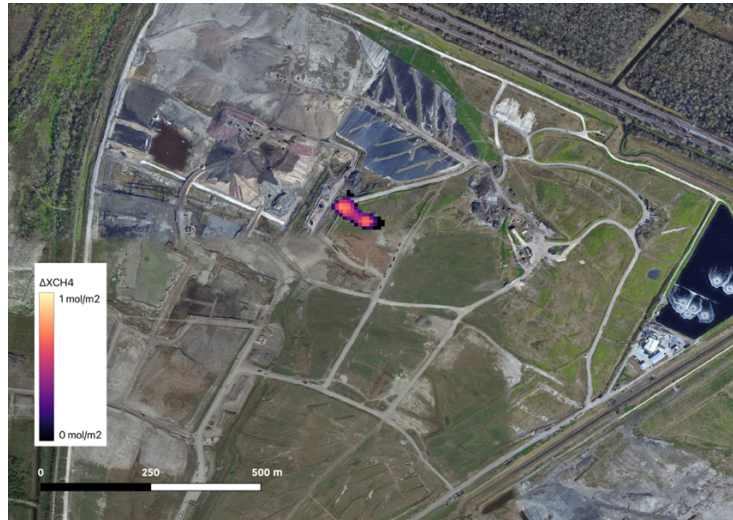
Figure 7.7 Possible methane plume April 25 th 2022. The background image is provided by Google Earth.
