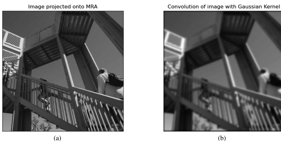
FIG. 5. Illustration of the convolution process in VAMPyR. (a) Original image projected onto the Multiresolution Analysis (MRA). (b) Resulting image after performing convolution with a Gaussian Kernel, leading to smoothing or blurring of the original image.
