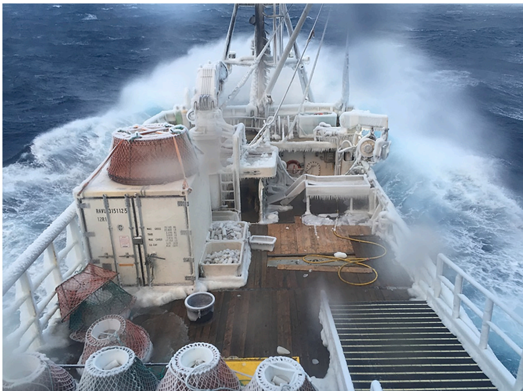
Fig. 1. Anti-icing measure on the M/S Northeastern traveling in sea-spray icing conditions (Birkeland, 2023).
