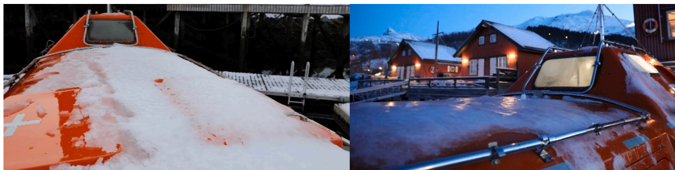
Fig. 12. Ice on the roof after deicing test Miriam lifeboat, March (left) and January (right).
