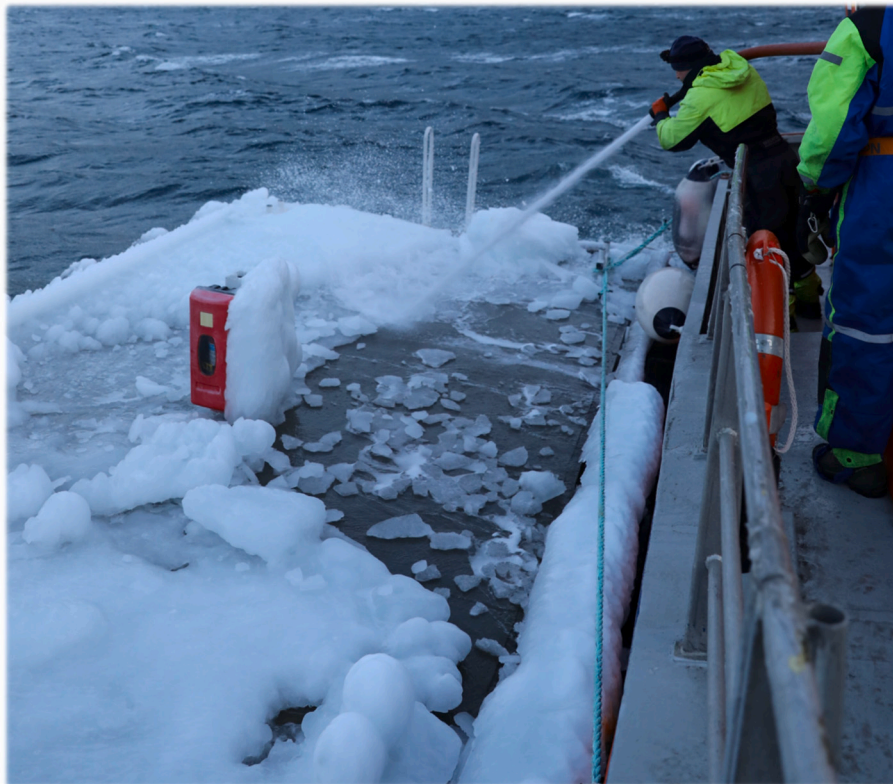
Fig. 18. Ice break-up when removing ice with a fire hose at full capacity.
