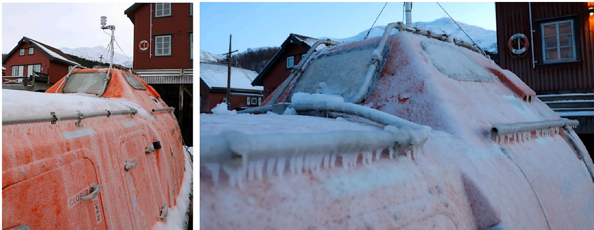
Fig. 8. Ice layer on the Miriam lifeboat prior to tests, March (left) and January (right).
