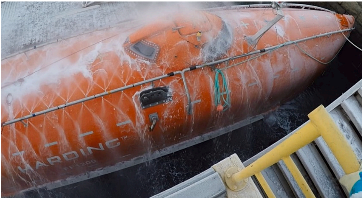
Fig. 15. Deicing of the Palfinger FF1200 lifeboat (Sundsbø and Jacobsen, 2018).
