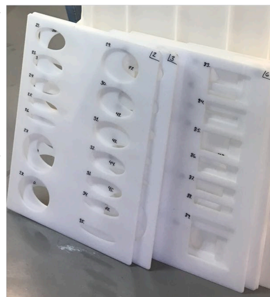
Fig. 3. Escape gap templates. Left: dimensions of rectangular and elliptic escape gap templates used in the fall-through experiments showing the values of the parameters A and B (in mm). Parameter B for the elliptical escape gaps and parameter A for rectangular escape gaps are shown as a corresponding size range. Right: photograph of an example of escape gap templates used during the laboratory experiments.
