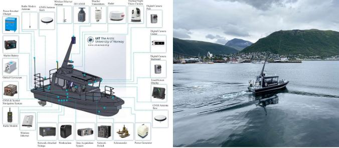
Fig.7. The equipped sensors in the autonomous ship "Ymir" and the sea trail experiment in Tromsø area.
