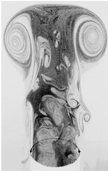
Figure 1. Example of material fluid deformation: A cross section of a laboratory thermal plume as visualized by condensed water distributions in gray (courtesy of Anna Gorska and Szymon Malinowski, University of Warsaw).
