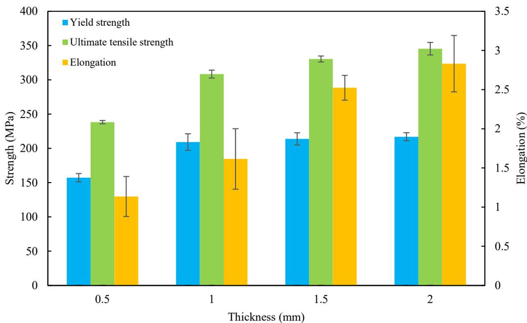
*Fig. 2 Variation of average yield strength, ultimate tensile strength, and elongation at fracture for different thickness of the samples. Error bars indicate one standard deviation.*
