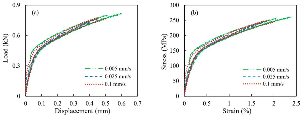
Fig. 6 Strain rate variation for the samples with 0.5 mm thickness a) Load-Displacement diagram b) Stress-Strain curve.
