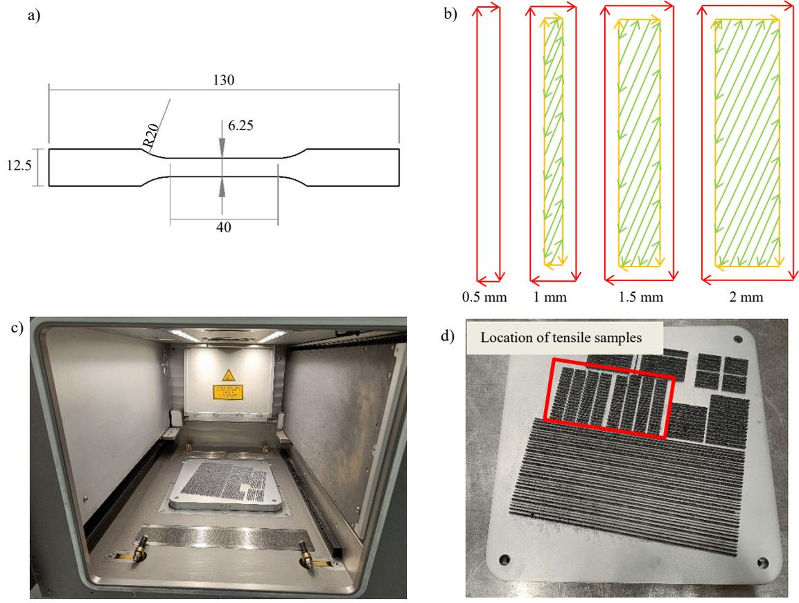
Fig. 1 a) Tensile sample geometry b) Schematic of scanning pattern for different thickness sizes in the gauge part of the samples c) Picture of the built plate inside of the working area of the machine d) Picture of the build plate after cutting down the samples.
