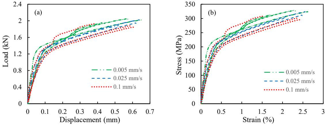
Fig. 5 Strain rate variation for the samples with 1 mm thickness a) Load-Displacement diagram b) Stress-Strain curve.
