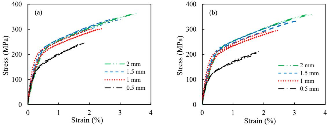
Fig. 4 Stress-Strain curve for variation of the thickness a) Nominal cross section b) Measured cross section.
