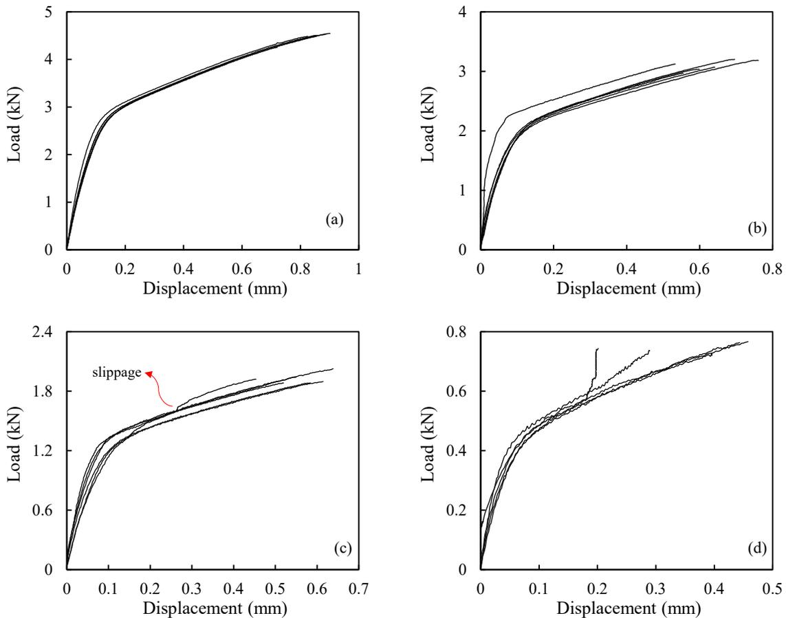
*Fig. 3 Load-Displacement diagram for all samples: a) 2 mm thickness samples b) 1.5 mm thickness samples c) 1 mm thickness samples d) 0.5 mm thickness samples.*
