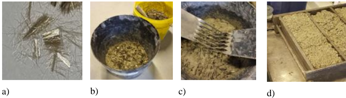
Figure 2: a) BB short fibers; b) concrete layer with fibers on its surface; c) mixing; d) fresh fiberconcrete cubes in moulds on the vibrating table.
