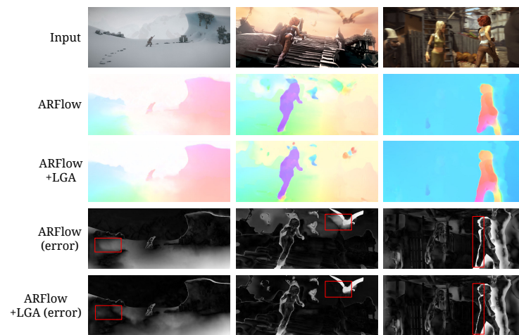
Figure 7. Results of unsupervised optical flow prediction on the MPI Sintel final-pass benchmark [40]. The first row shows the input samples, and the next two rows show the estimated flow for ARFlow [26] and LGA with ARFlow. The last two rows visualize the incurred EPE-all errors for each of the methods on the final pass. Notable differences are highlighted by red boxes.
