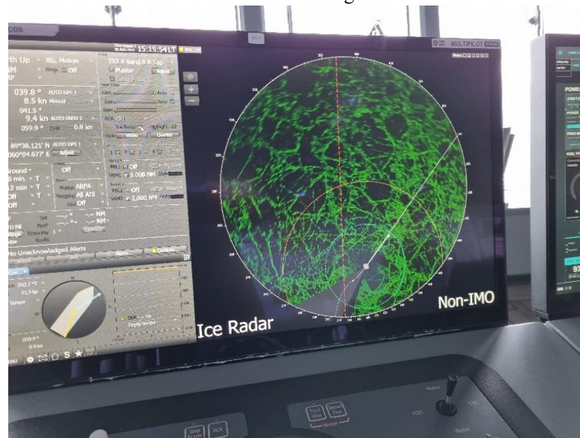
Figure 8 Ice Radar onboard LCC
