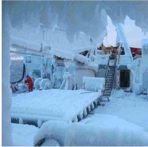
Fig. 1 A case of ice accumulation event in Arctic regions (Kubat I, 2005).
