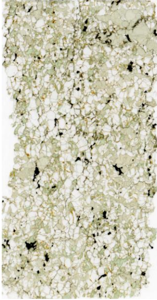
BVC-29 Type: Coarse granular ol: 55% opx: 35% cpx: 9% spl: 1%
