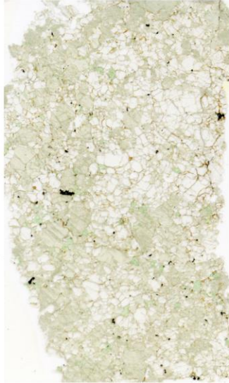
BVC-24 Type: Coarse granular with olivine and opx porphyroclasts ol: 78% opx: 17% cpx: 4.8% spl: 0.2%
