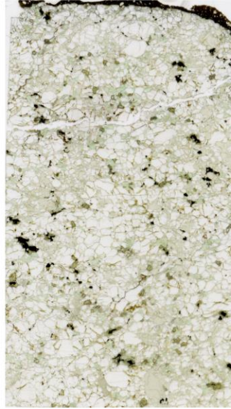
BVC-30 Type: Coarse granular ol: 57% opx: 35% cpx: 7% spl: 1%
