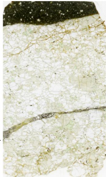
BVC-32 Type: Coarse granular with olivine and opx porphyroclasts ol: 65% opx: 30% cpx: 2.9% spl: 0.1%
