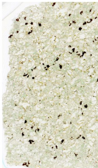
BVC-23 Type: Granular ol: 45% opx: 37% cpx: 16% spl: 2%
