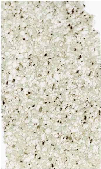
BVC-20 Type: Coarse granular ol: 51% opx: 35% cpx: 10% spl: 4%
