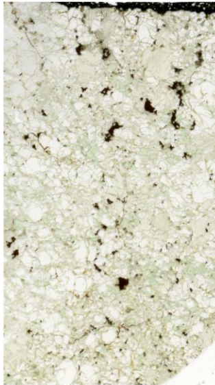
BVC-01 Coarse granular ol: 55% opx: 33% cpx: 10% spl: 2%
