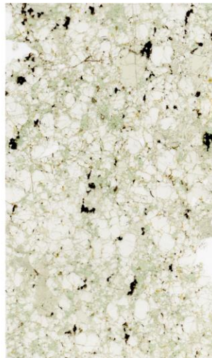
BVC-04 Coarse granular ol: 66% opx: 25% cpx: 7% spl: 2%
