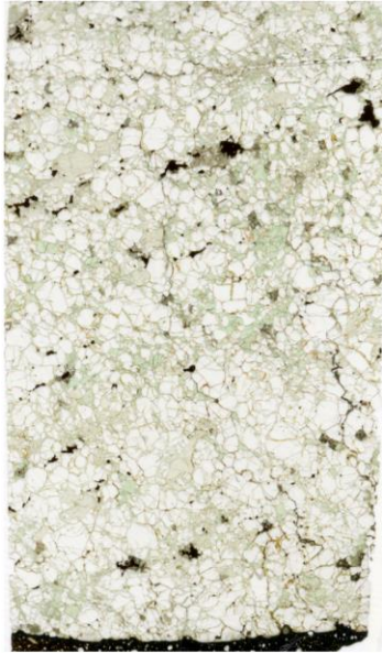
BVC-08 Type: Coarse granular ol: 65% opx: 24% Cpx: 10% spl: 1%
