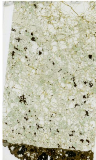
BVC-40 Type: Coarse granular with olivine porphyroclasts ol: 45% opx: 38% cpx: 15% spl: 2%
