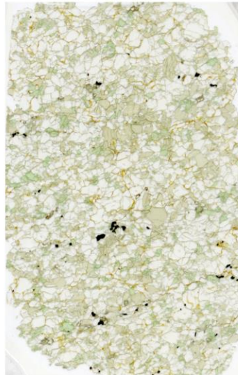
BVC-38 Type: Coarse granular ol: 60% opx: 30% cpx: 9.5% spl: 0.5%
