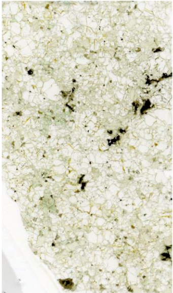
BVC-26 Type: Coarse granular ol: 60% opx: 34% cpx: 4% spl: 2%
