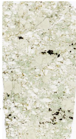
BVC-06 Type: Coarse with opx porphyroclasts ol: 56% opx: 31% cpx: 11% spl: 2%
