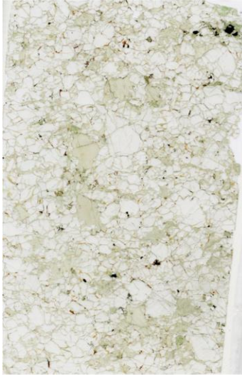
BVC-24 Type: Coarse granular with olivine and opx porphyroclasts ol: 78% opx: 17% cpx: 4.8% spl: 0.2%
