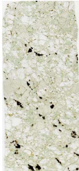
BVC-02 Coarse granular ol: 50% opx: 40% cpx: 8% spl: 2%
