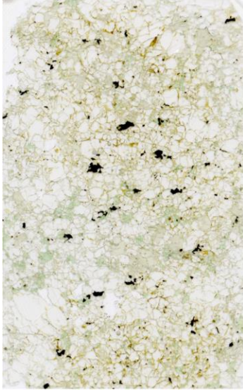
BVC-17 Type: Granular with olivine porphyroclasts ol: 65% opx: 25% cpx: 18% ?? spl: 2%
