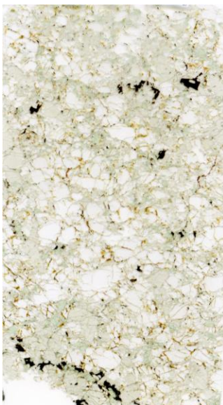
BVC-22 Type: Coarse granular ol: 55% opx: 39% cpx: 4% spl: 2%
