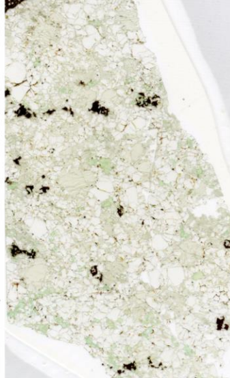
BVC-19 Type: Coarse granular with olivine and opx porphyroclasts ol: 61% opx: 30% cpx: 7% spl: 2%
