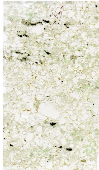
BVC-21 Type: Coarse granular with olivine porphyroclasts ol: 65% opx: 25% cpx: 9% spl: 1%
