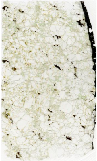
BVC-27B Type: Coarse granular ol: 75% opx: 20% cpx: 4% spl: 1%
