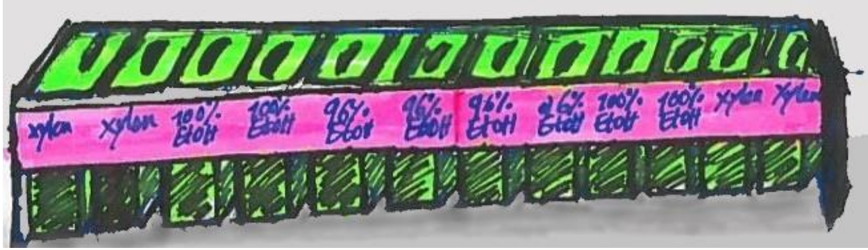
Figure 19: Depicting the deparaffinization (left) and dehydration (right) with decreasing and increasing ethanol solution, sequentially.
