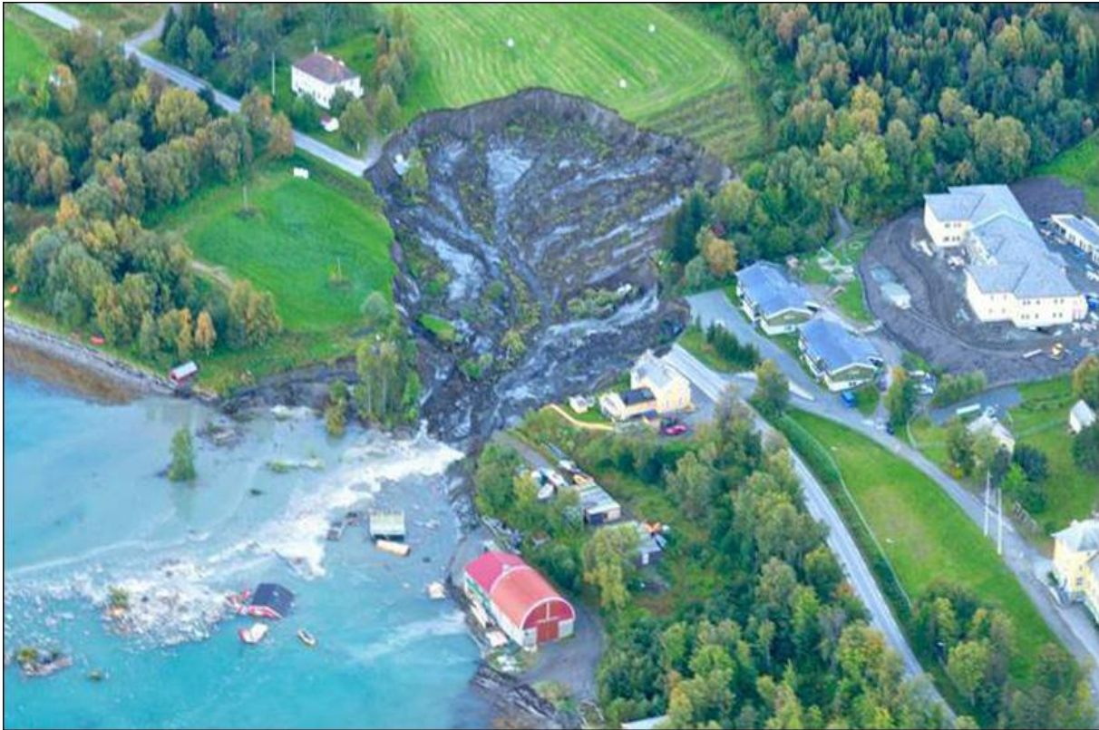
Figure 1.11: Photograph showing the outline of a mudslide in marine clay deposits near Lyngseidet. This slide occurred in September 2010 (photo by Andrea Taurisano/NVE).
