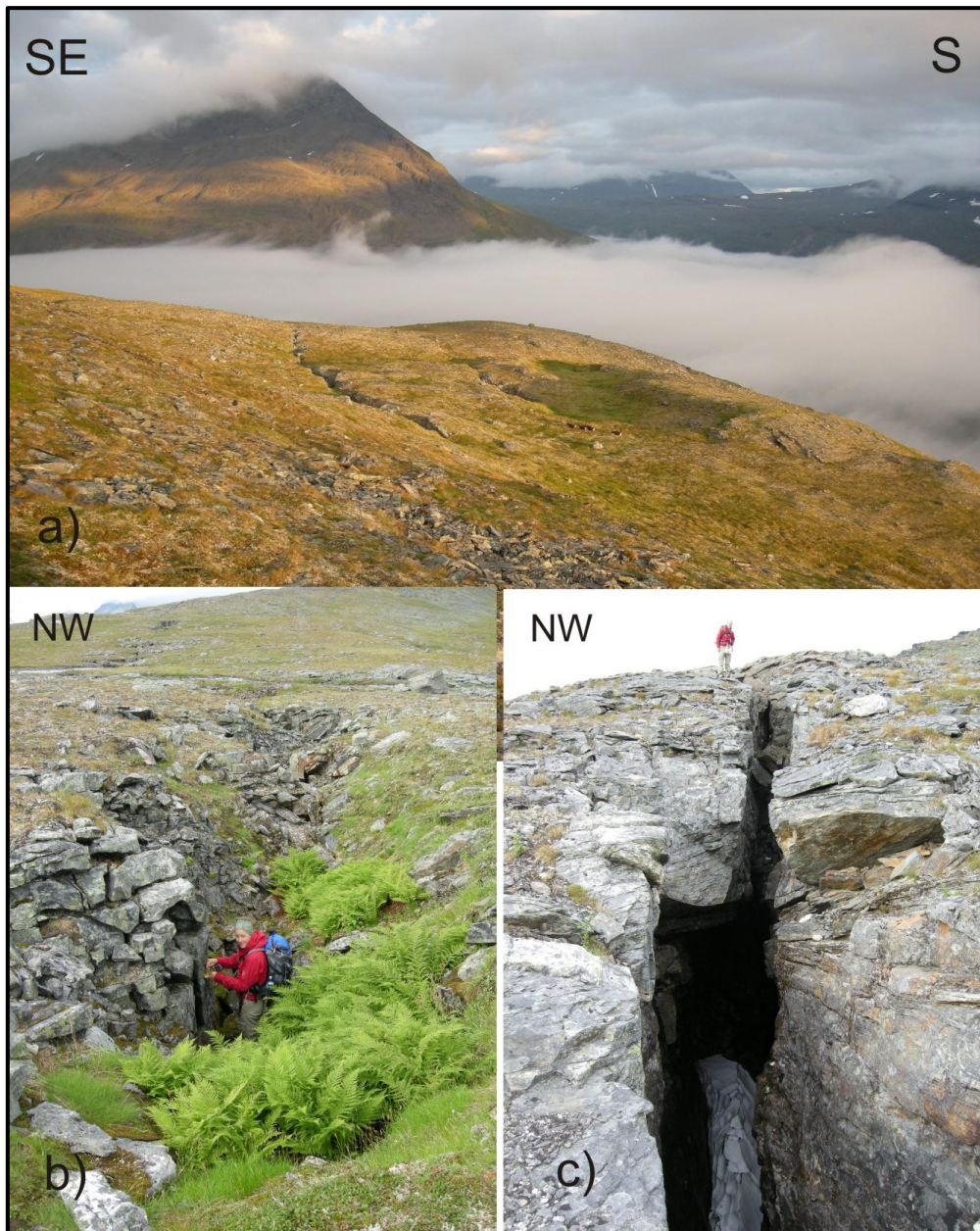
Figure 4.13: Photos showing various fractures in the studied RSF area: (a) Extensional fractures showing a slight bending geometry towards NW (b) Some are vegetated with ferns (c) Open fractures in Domain II, above the main rock slope failure area. The deepest ones have almost an “A” shape, narrow on top and widening deeper; they are so deep and cold that the snow does not melt in them 20 meters down.
