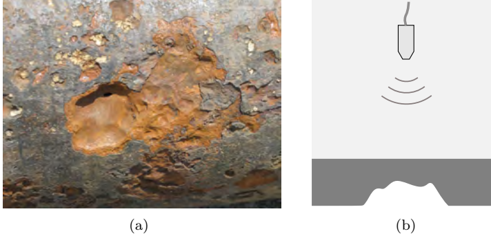
Figure 5.1: (a) Example of pitting corrosion. (b) Measurement geometry for outside pitting corrosion.
