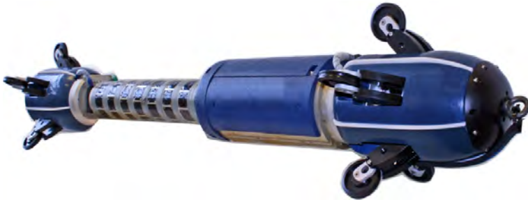
Figure 1.1: The inspection robot used by BIT to inspect water distribution networks. 64 ultrasound transducers are to measure the inside topography and the remaining wall thickness of the pipe. Photo: BIT
