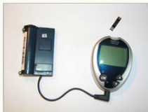
Figure 2. The Bluetooth transmitter (left) sends glucose measurements to the phone as soon as the test strip is extracted from the glucometer.
