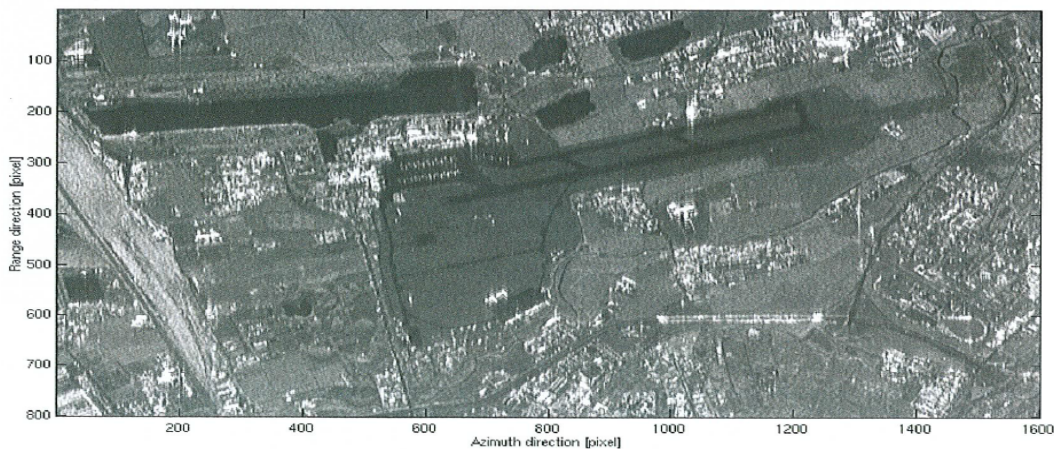
Figure 2.6: Average of multiple ERS SAR images of the Linate airport. The speckle is suppressed on the homogeneous fields nearby the airport (figure taken from [Ferretti et al., 2007]).
