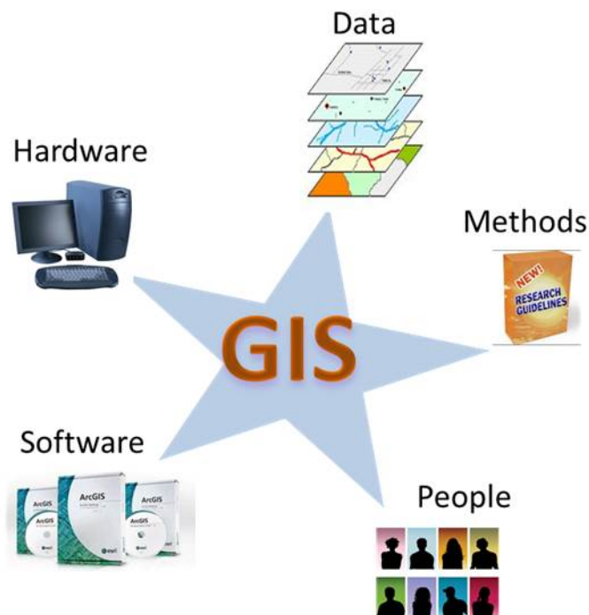
Figure 6. Main characteristics of GIS. Hardware is the computer, printer, network etc.; the software provides the tools needed for storing, visualizing, analysing etc.; the data consist of both geo-referenced data and related attribute data, methods are available tools like guidelines, standards, applications and procedures for handling the data; and people are needed to manage the system and develop plans for applying the technology (after Bernhardsen 2006).
