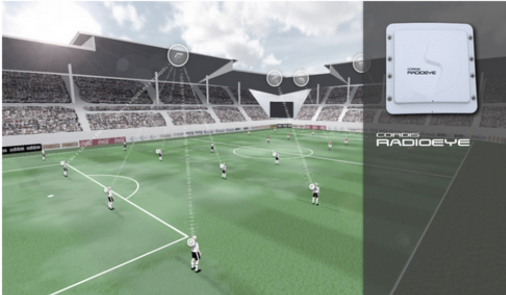
Figure 2.3: Overview of the ZXY system with receivers placed around the pitch, and players wearing sensors. Image from zxy.no
