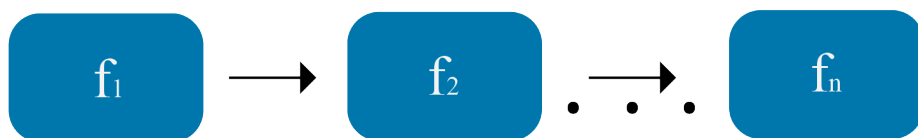
Figure 4.4: Functions chained where the output are sent as input to the next function
