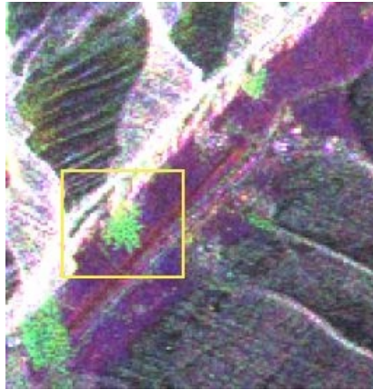
Figure 5.2: Image containing avalanche debris fields used in the green channel, causing avalanche debris fields to show as green. Image: [Wiesmann et al., 2001]
