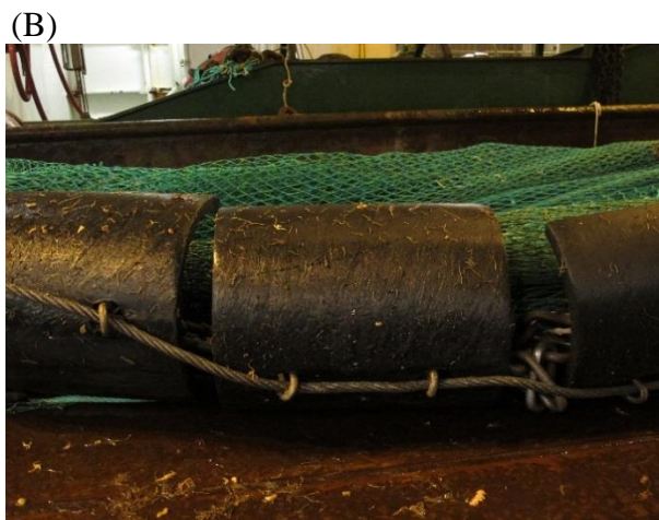
Figure 2.6 The semicircular spreading gear, from behind (A) and from the front (B).
