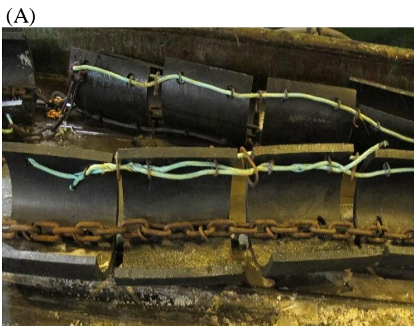
Figure 2.6 The semicircular spreading gear, from behind (A) and from the front (B).
