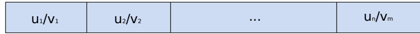
Figure 5.1: Memory layout for the ALS-CUDA algorithm. Both weight matrices are stored vector-wise.
